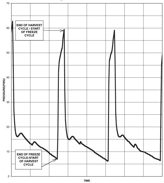
The chart above shows the low side pressure changes through the cycles of a CLR2060 unit. It shows that during a harvest cycle, the low side pressures climb to nearly 60 psig. When the freeze cycle starts, the pressure quickly drops to approx. 17 psig and throughout the freeze cycle it continues to slowly drop to approximately 7 psig just before the harvest cycle.
